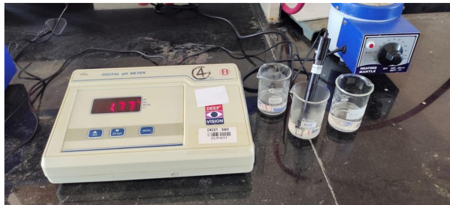
Figure.5. pH Sensor Output Comparison with Standard Digital Meter
